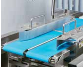
Spacing conveyor with motorised infeed guides
